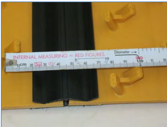
(Example: Allowable distance between two rows of studs at the joint)
